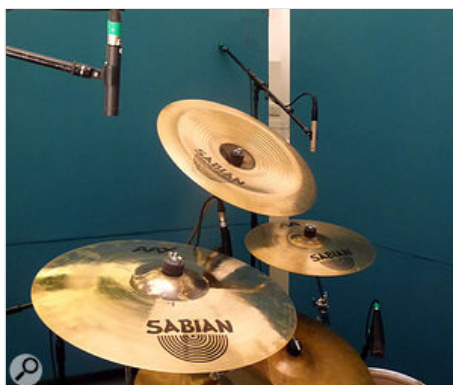
5. The nearest Neumann KM184 is used for paired cymbal miking, positioned to ensure that the nearest crash and large china next to it are as evenly balanced as possible. The furthest crash cymbal has been allocated an individual cymbal mic.
