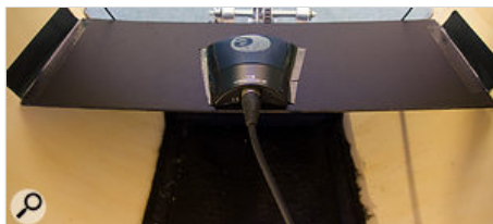
2. A Sennheiser e901 'attack' mic placed on some strong corrugated card secured horizontally across the kick drum around a third of the drum's height. The cartridge is about six inches below the batter head contact area.
