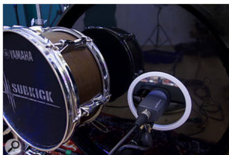
1. Three-mic Kick Trick, featuring a Yamaha Subkick outside the resonant head; a Sennheiser e602 placed half-in/half-out of the port; and a Sennheiser e901 (see picture 2) as an internal 'attack' mic.
