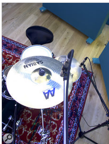
4. Neumann KM184 mics used on the crashes, placed in such a way that the cymbals prevented some of the hat's and snare's high frequencies reaching the mic directly.
