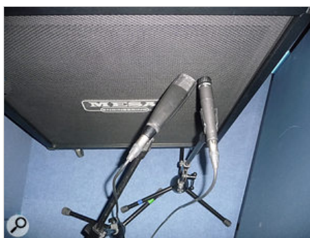
8. The dual-mic technique used on guitar cabs, with phase-aligned SM57 and MD421 dynamic mics.
