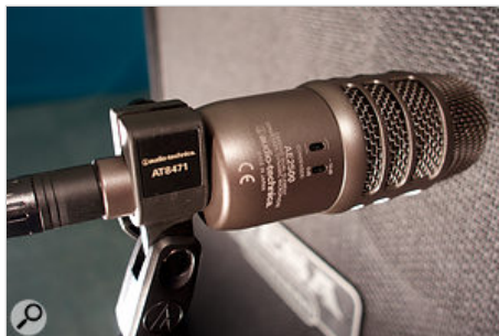
9. The Audio Technica AE2500 is a dual-diaphragm mic that consists of phase-aligned dynamic and condenser capsules within the same housing.
