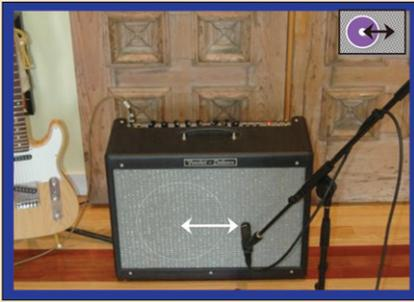
Fig. 2: Moving off center of driver
